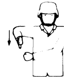
LOWER THE BOOM AND HOLD THE LOAD
