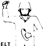
LOCK THE CRAWLER BELT ON SIDE INDICATED BY RAISED FIST - TRAVEL OPPOSITE CRAWLER BELT IN DIRECTION INDICATED BY REVOLVING FIST LEFT TURN
