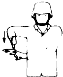
LOWER THE BOOM AND RAISE THE LOAD
