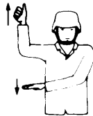
RAISE THE BOOM AND LOWER THE LOAD
