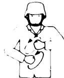
TRAVEL BOTH CRAWLER BELTS IN DIRECTION INDICATED BY REVOLVING FISTS
